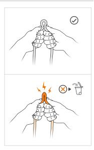
Do a tactile inspection of the core for the full length of the rope (hard spots, swelling, soft or crushed areas...).
