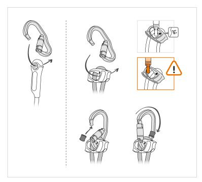
• Reinstall the connectors Verify that the connector is correctly positioned in the rope clamp.
