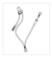
• Check the condition of the rope at the harness attachment holes and at the ends of the lanyard.
