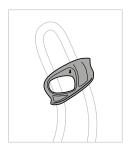
• Check the condition of the rope clamp (marks, wear, cracks, deformation, corrosion...).
