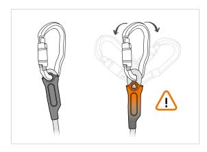
• Verify that the plastic protective sleeve correctly positions the connector
