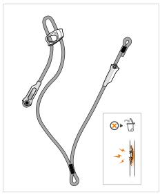
• Look for wear and damage on the sheath due to use (cuts, fuzziness, chemical residues...)
