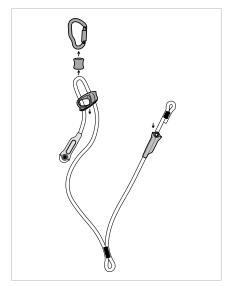
• Remove the connectors from the individual strands. Remove the protective sleeve from the lanyard side, and the rope clamp, in order to check the hidden areas.
