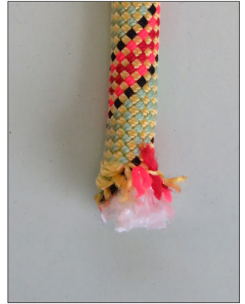
• Damaged rope end
