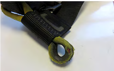
• Damaged attachment point
