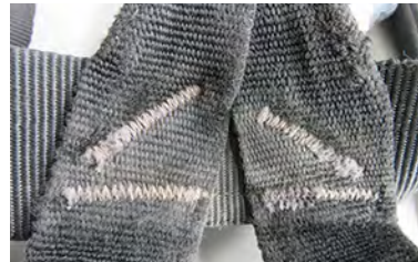
• Damaged safety stitching
