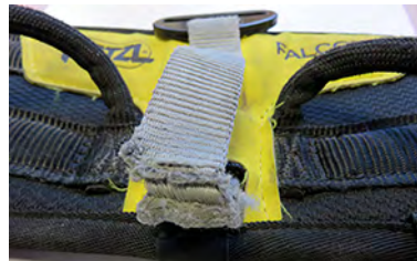
• Damaged attachment point
