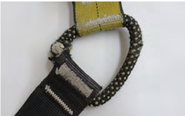
• Damaged attachment point
