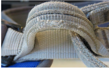
• Worn tie-in point
