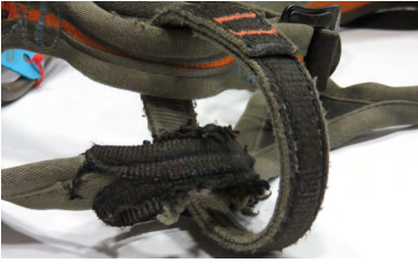
• Worn tie-in point
