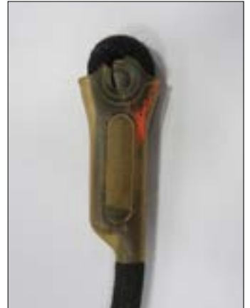
• Damaged plastic sleeve
