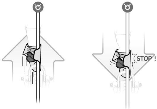
Installing and removing the rope
