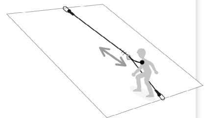
7. EN 358: 2018 belt for work positioning and restraint
