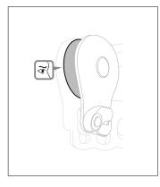
• Check the condition of the sheaves (marks, deformation, cracks, corrosion, wear, absence of foreign bodies...).
