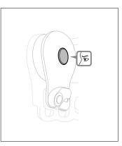
• Check the condition of the rivets (marks, deformation, cracks, wear, corrosion, absence of play...).
