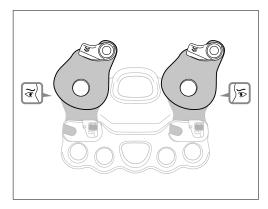
• Check the condition of the side plates (marks, deformation, cracks, wear, corrosion).
