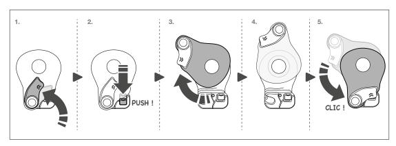
• Check the condition and function of the locking system (marks, deformation, dirt, effectiveness of the return spring(s)).
