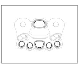
• Check the condition of the attachment holes (marks, deformation, cracks, wear, corrosion...).
