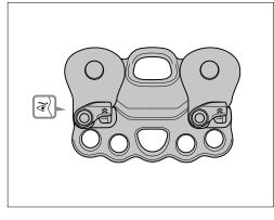
• Check the general condition of the product (marks, deformation, cracks, wear, corrosion...).
