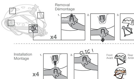
Removal/installation of the liner
