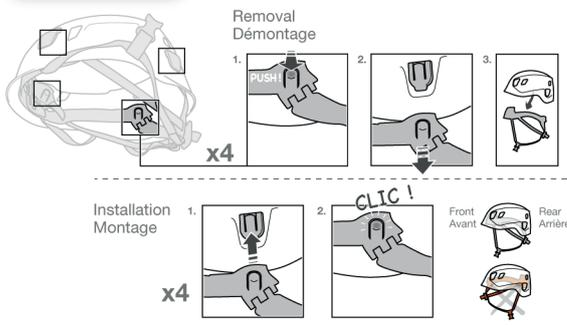
Removal/installation of the liner
